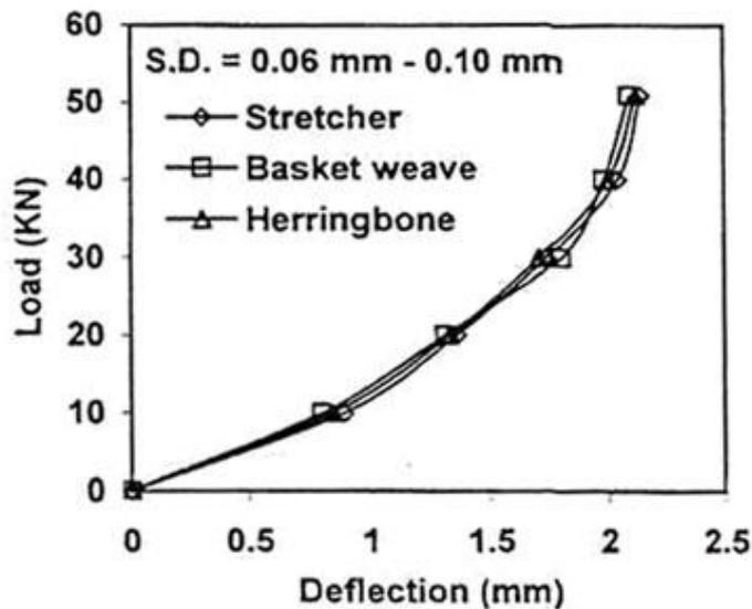
Figure 1. Deflection of block pavement against load increasing [2].
