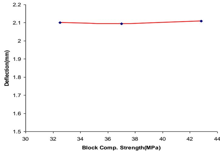
Figure 7. Effect of Block Strengths on behavior of Block Pavement.
