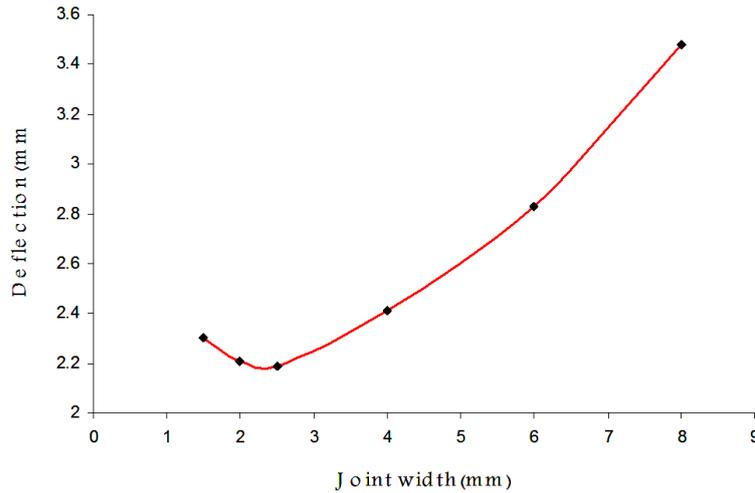
Figure 5. Pavement deflections with varying joint width.
