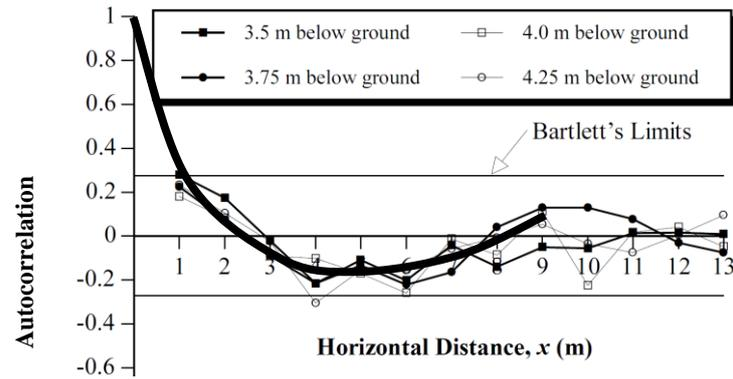
Figure 10. Variation of ACFs for  $q_c$  and fitted deterministic trend with horizontal distance (Modified from Jaksa et al. [3]).
