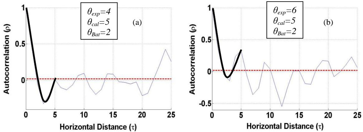
Figure 8. Variation of ACF with lag distances for a)  $\theta=4$  b)  $\theta=6$ .
