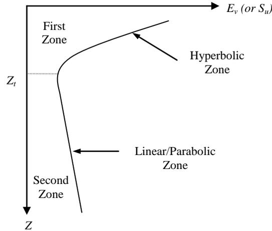
Figure 2. Schematic shape for variation of vertical stiffness modulus [4].
