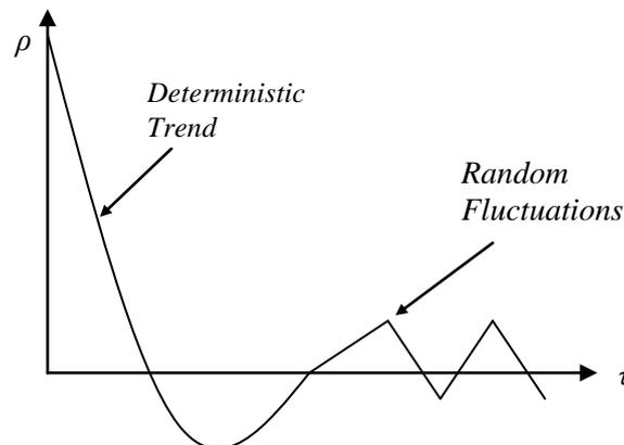
Figure 7. Schematic shape for the variation of ACF with lag distance.
