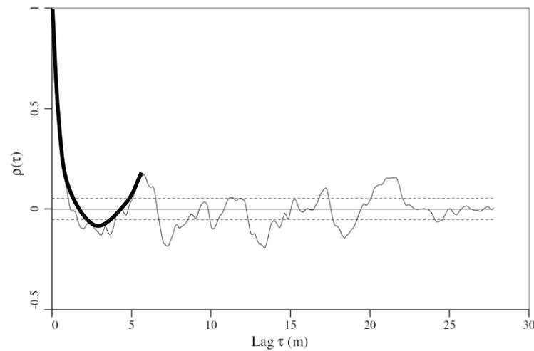
Figure 11. ACF for a  $q_c^{0.74}$  record of length 27.8 m and fitted deterministic trend (Modified from Fenton [16]).
