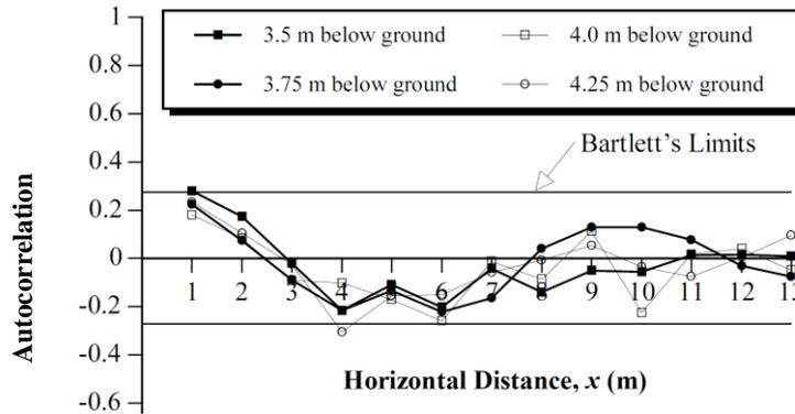
Figure 4. Variation of ACFs for  $q_c$  with horizontal distance [2].
