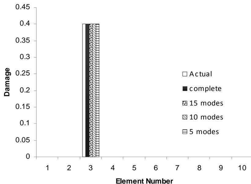
Figure 3. Cantilever beam with damage at Element 3: effect of incompleteness of mode shape data on damage detection data in Scenario 1.
