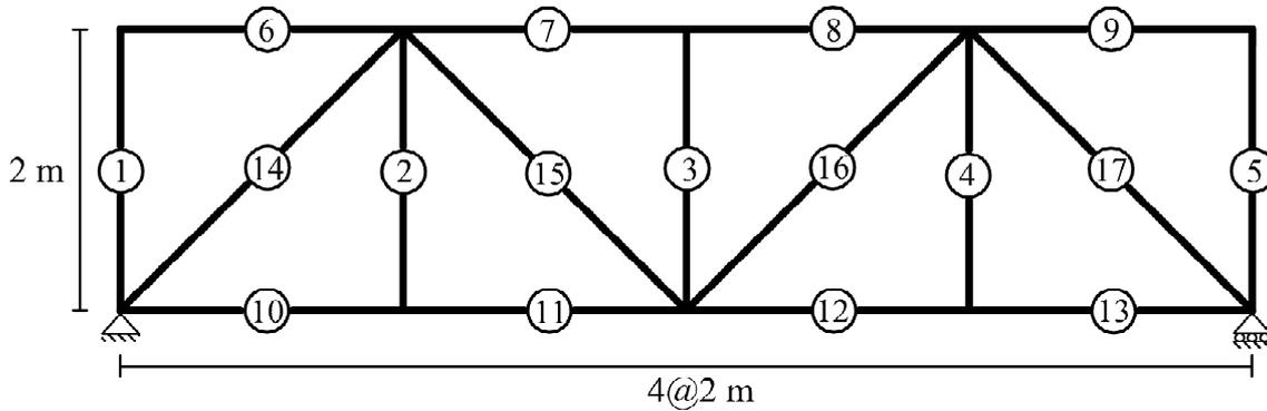
Figure 6. The finite element model of a truss having 13 elements.
